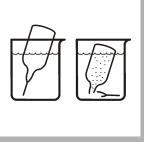
2. Prepare the blank: Pour at least 40 mL of deionized water into a 50-mL beaker. Fill an AccuVac Ampul with deionized water. Keep the tip immersed while the Ampul fills completely.
