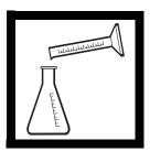
**4.** Use a graduated cylinder or pipet to measure the sample volume from *Table 1* or *Table 2*. Transfer the sample into a clean 250-mL Erlenmeyer flask. Dilute to about the 100-mL mark with deionized water, if necessary.
