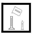
1. Select a sample size and an EDTA Titration Cartridge corresponding to the expected calcium as calcium carbonate (CaCO<sub>3</sub>) concentration. Use Table 1 for concentrations in mg/L or Table 2 for concentrations in German degrees of hardness (G.d.h.).
