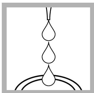
**6. Use a pipet to add 0.4 mL of Ferric Ion Solution into each sample cell.**
