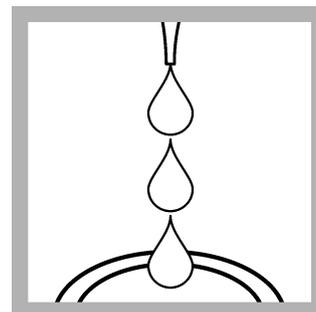
**4. Use a pipet to add 0.8 mL of Mercuric Thiocyanate Solution into each sample cell.**
