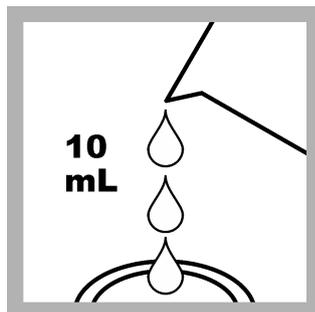
**3. Prepare the sample:** Fill a second sample cell with 10 mL of sample.
